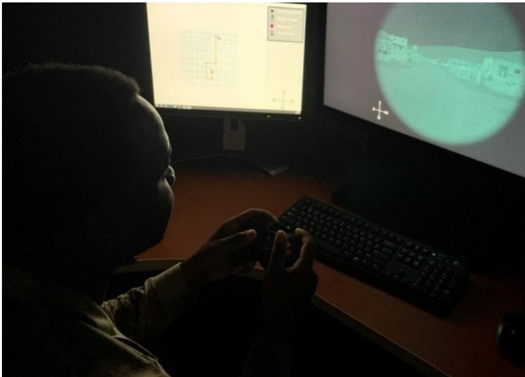
Figure 2-1: Experimental set-up. A Soldier completes a navigation route by using two computer screens. The primary computer screen displayed the NVD sensor feed, and an adjacent, secondary computer screen displayed the “printed” map.
